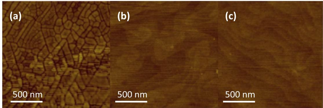
**Figure 4.** Surface morphology of sample A(a), C(b) and H(c), characterized by the tapping mode AFM. The scan scales are all  $2 \times 2 \mu\text{m}^2$  and the RMS roughness are 0.40, 0.20 and 0.19 respectively. The z-scale is 5 nm.
